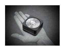
We also developed a high-performance brushless and gearless servo motor. As is well known, brushless motors have many good points, which are preciseness, smoothness, quietness and low-power consumption. Keigan Motor, whose maximal torque is over 2.6 lbf·in (0.3N·m) with less than 10W power consumption, rotates precisely, smoothly, and quietly. It can be controlled to any angle you like with accuracy of  $0.05^{\circ}$ .
